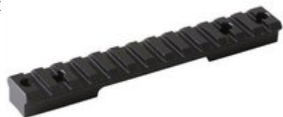
Underside of base is cut out to accommodate receivers with right- or left-hand ejection ports. Aluminum models machined from 6061 T6 billet for maximum weight reduction. Matte, black, anodized finish blends with most factory finishes.
